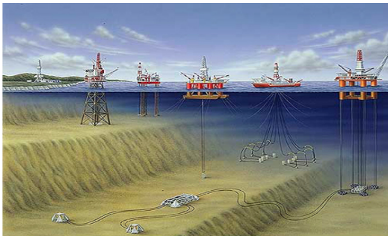
Left to right: onshore platform; fixed platform; jackup rig; semi-submersible;
